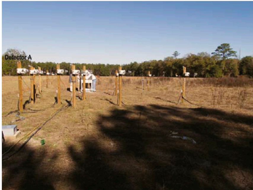
FIG. A3. A photograph of the layout of the LPM (optical disdrometers) network. The origin of the network is taken to be at detector A indicated at the left. Arm 3 is the leftmost line of detectors. The white box is the 2DVD toward the left of center.
