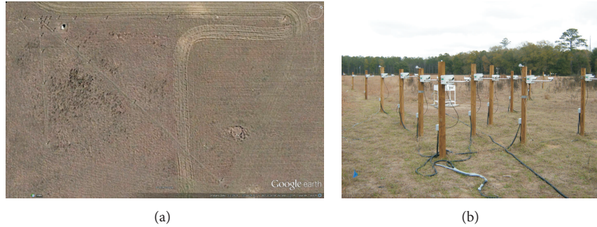
FIGURE 2: Pictures of the disdrometer array. (a) shows an overhead view of the site (as of March 1, 2014). The shadows of the LPMs can be identified by looking closely. The picture is aligned to replicate the general geometrical alignment shown in Figure 1; detector “A” is in the upper-left. The white object in the center of the box formed by detectors K, L, S, and T is a 2-dimensional video disdrometer (not used in this study). (b) displays part of the array from ground level. The first detector in the foreground is detector “A,” with the 2-dimensional video disdrometer visible in the background. All detectors are mounted nominally 1.75 meters off of the ground.
